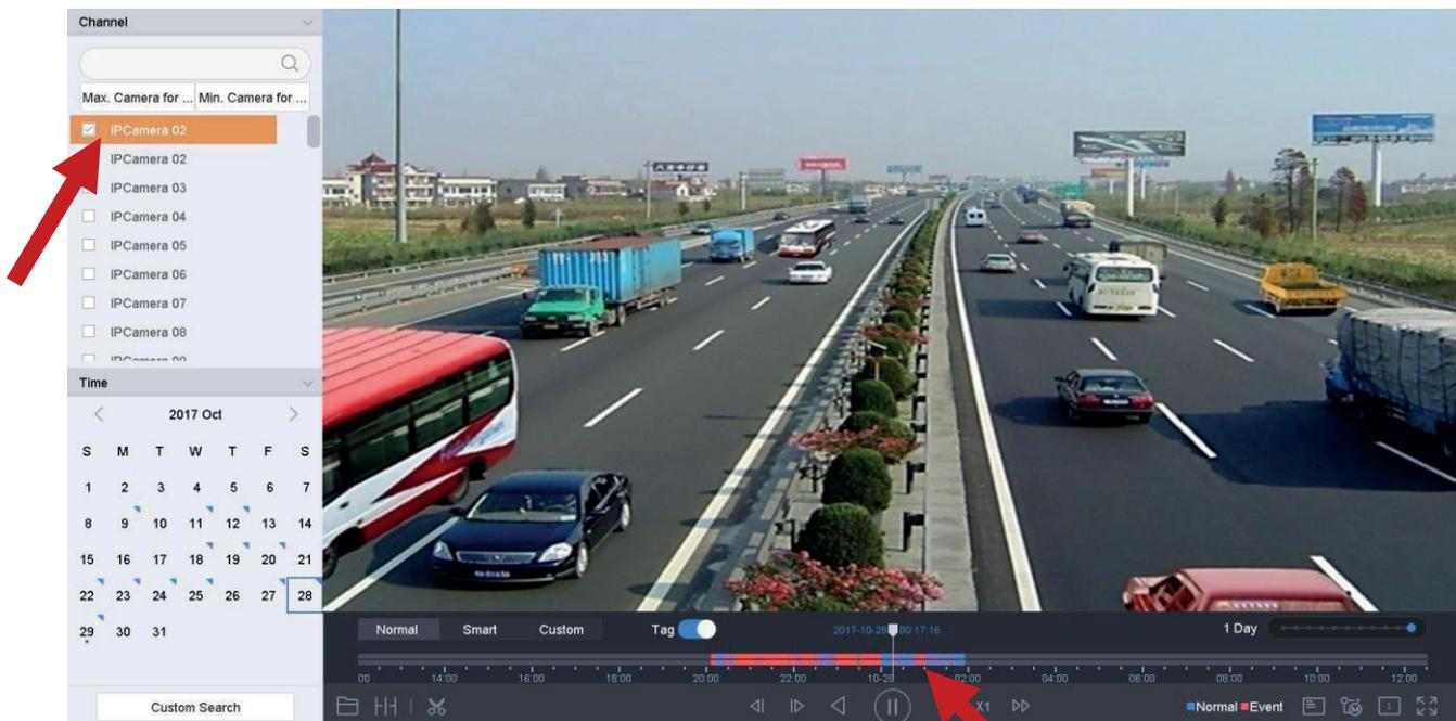
4. The Screen above should then appear, allowing you to select the cameras of interest from the left-side of the screen by ticking the boxes, these cameras will then show on a split-screen.
